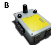
Portable Train Detector PT-0501 Magnetically attached to track
