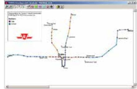
The system map module of MOWIS provides a graphical display of the entire rail system together with outstanding track defects.
